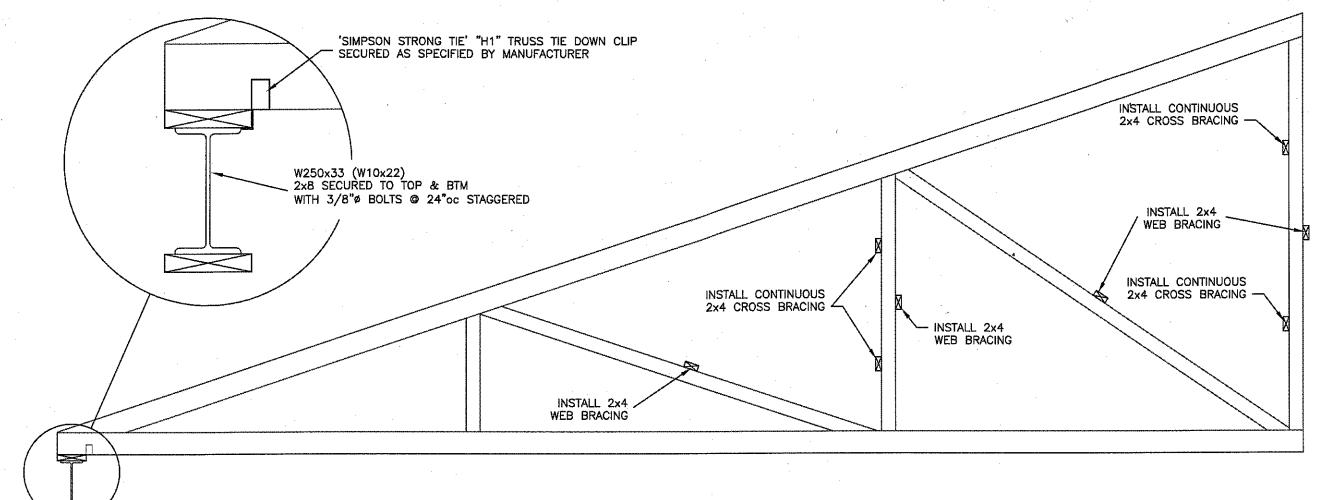
EXISTING TRUSSES WITH NEW BEARING SUPPORT AND WITH BRACING TO BE INSTALLED
